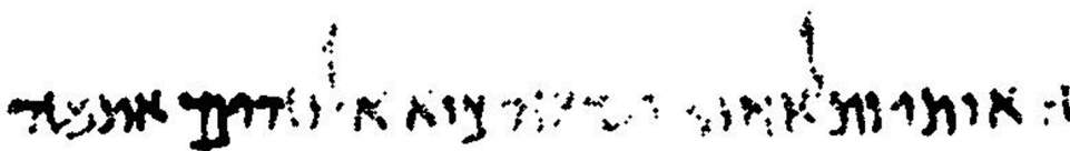
Figure 7.4: An example of when opening with an elliptical kernel size 3x3 is performed on a DSS image that has undergone Otsu thresholding. Some of the letters are almost completely removed. DSS image gotten from: [4]
