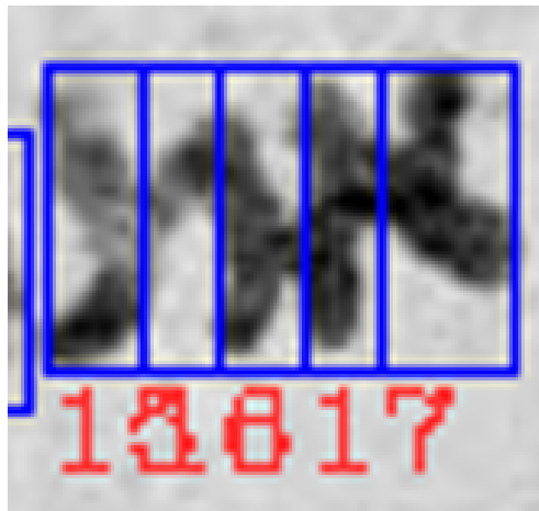
(a) The letters between number 15 and 17, found in this Figure 7.7, were unsuccessfully segmented.
