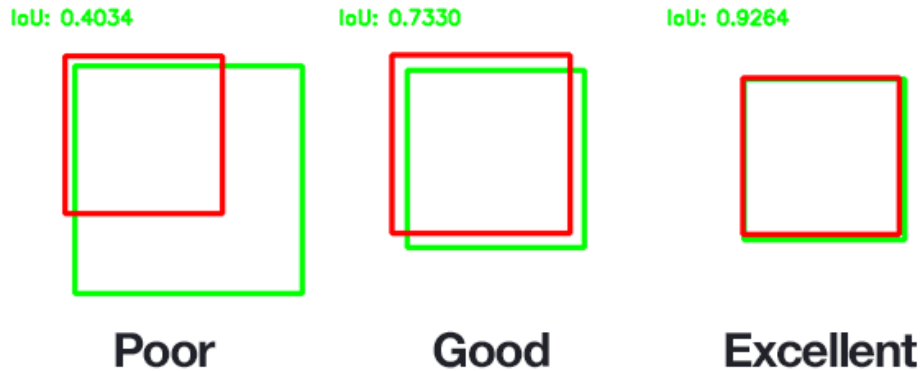
Figure 3.4: Figure that shows an example of a poor, good and excellent IoU score. Source: [23].
