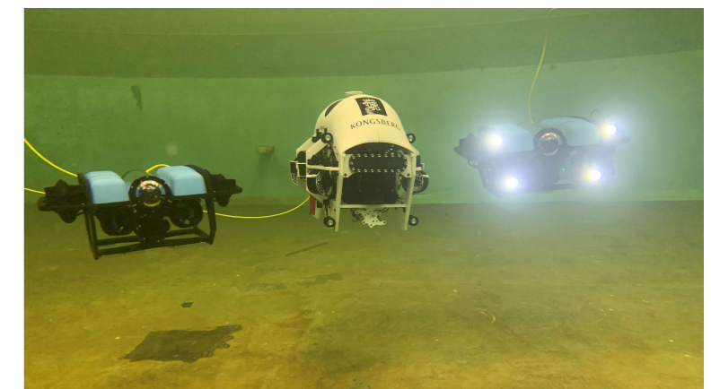
From left to right: BlueROV2 Heavy, Vortex Beluga Mk.2 and BlueROV2 Heavy modified at ITK
