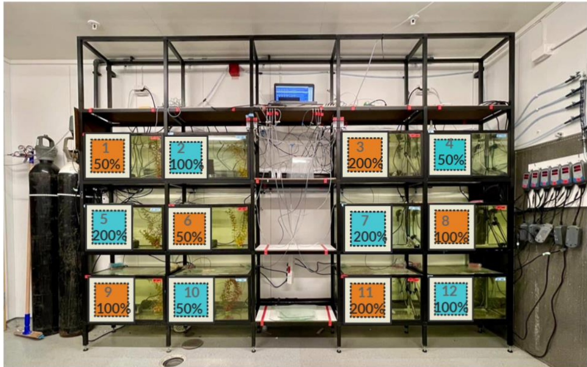
Figure 7: Set up of the experiment. Twelve tanks distributed on the shelf so that neither of the same treatments experienced the same position in the room. Oxygen and nitrogen-tanks to the left supplying hypoxic and hyperoxic aquaria, respectively. All plastic tubes connecting aquaria with gas are joint in a manually adjusted valve-station below the computer. Duplicated treatments resulting in six cold and six warm aquaria combined with three different oxygen treatments.
