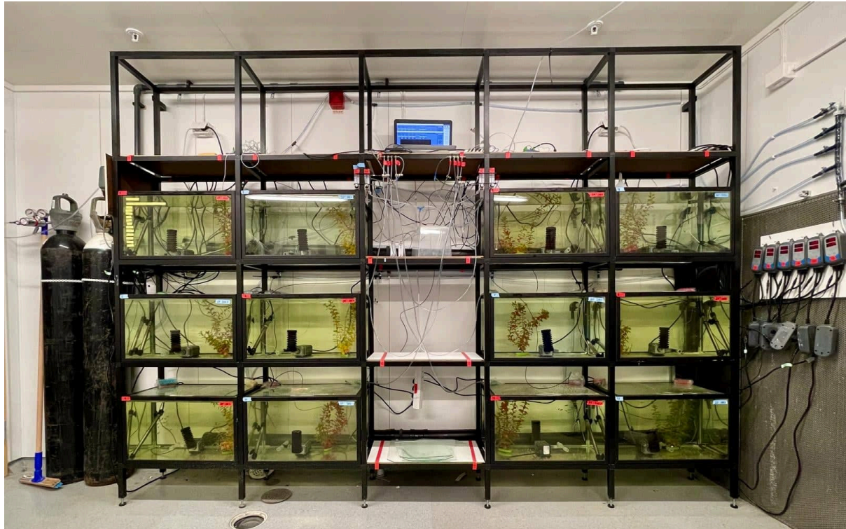
Figure 2.1 The experimental set up for the acclimation project. To the left, there are one tank of N 2 and one tank of O 2 used for adjusting the amount of dissolved oxygen in each tank. To the right, we see half of the Inkbird thermostats controlling the temperature of individual tanks. On the top, one laptop was used to monitor oxygen saturation of the 4 hypoxic and the 4 hyperoxic tanks, as well as temperature for all 12 tanks.
