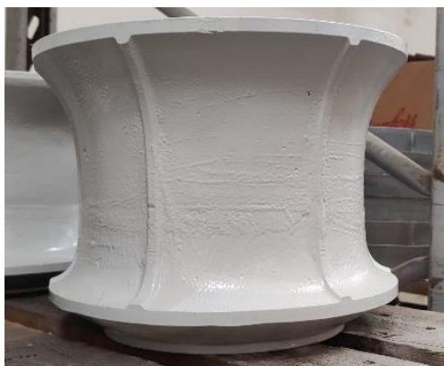
Figur 51 - PMH's ribbet kapstanhode
