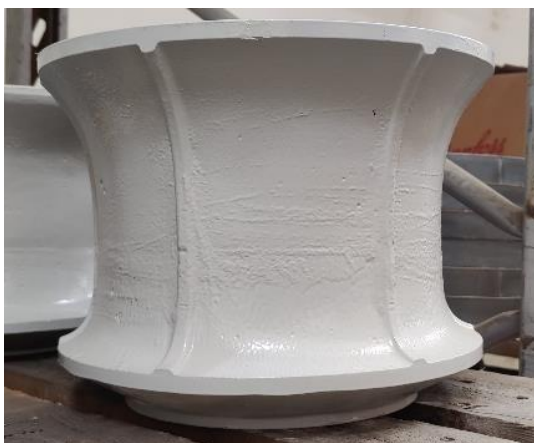
Figur 37 - PMH's ribbet kapstan
