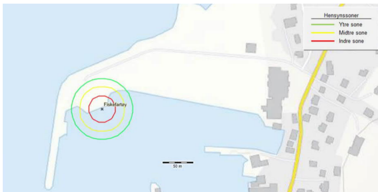
Figure 2.15: Safety zones for hydrogen bunkering in Ramberg [15].
