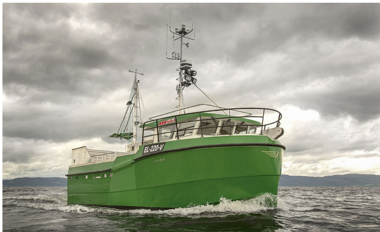
Figure 2.1: World's first hybrid fishing vessel, Karoline [18].
