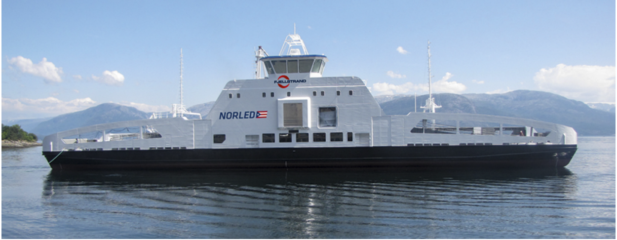
Figure 2.3: The worlds first electrical car ferry, MS Ampere [24]
