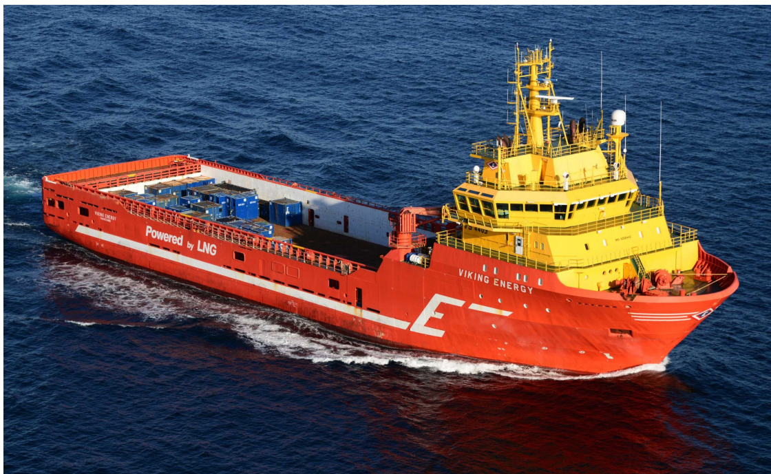
Figure 2.14: The worlds first LNG supply ship Viking Energy now being rebuilt into the worlds first ammonia supply ship [73].
