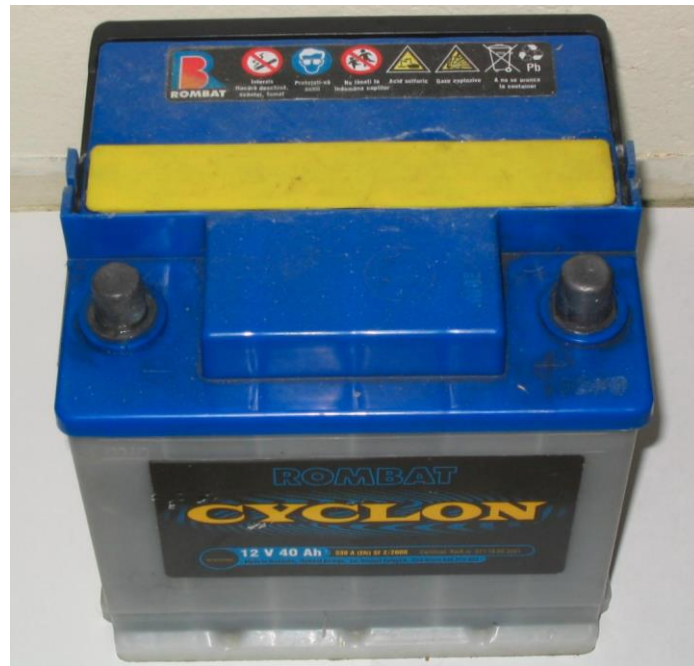
Figure 2.18: A traditional lead-acid car battery. Source: Wikimedia Commons [27]
