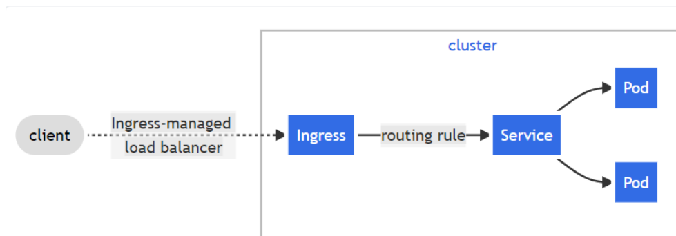
Figure 2.3: External access to services using Ingress [23]
