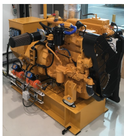
Figure 2.7: The marine diesel engine included in the hybrid power lab.
