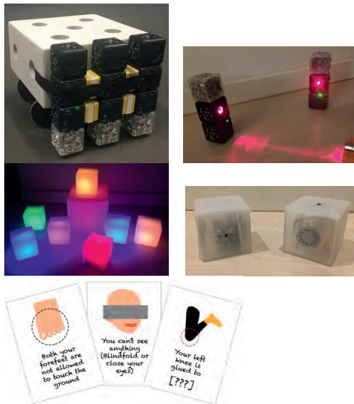
Figure 4: Move Maker elements: Proximity controlled mobile robot, laser lines, light cubes, music cubes and bodily precondition cards.
