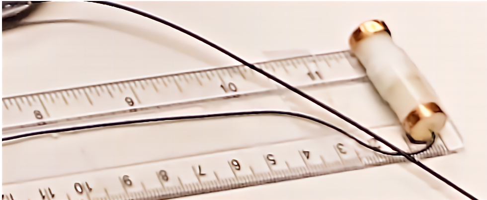
Figure 5.21: Dummy capsule with antennas made of copper foil and one coaxial cable for external connection to the backscatter switch
