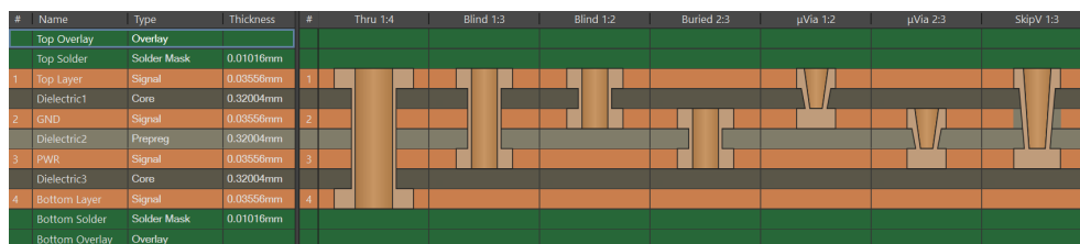
Figure 3.3: Typical stack up for a 4-layer PCB, with all possible via types for a 4-layer PCB
