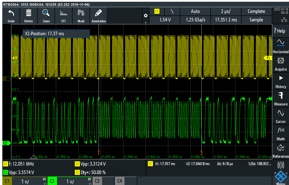
Figure 5.11: Closer view of the beginning of a row in READOUT mode. Shows that there are eight PPs of the training pattern.
