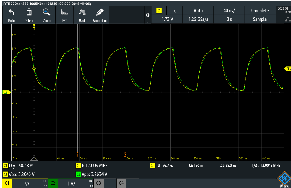
Figure 5.16: Comparison of the clock generated by the ams NanoBerry evaluation board in green and our 12 MHz MCO clock in yellow. They are almost exactly identical. The oscilloscope measures the frequency to 12.006 MHz, which is quite accurate. The cursors also verify this. The duty cycle is measured to 50.48 %, which is also good, as we ideally want 50.0 %.
