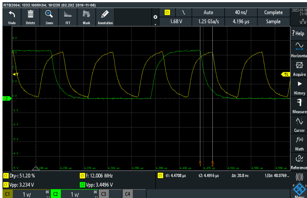
Figure 5.18: Data skewed 1 clock cycle to the left compared to the clock
