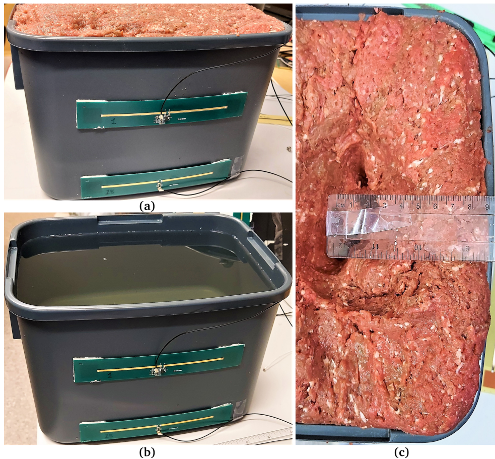
Figure 5.23: The bucket with the phantom materials used for testing. (a) shows the bucket with minced meat and (b) shows the bucket with the liquid phantom. (c) shows that the capsule is placed in the center of the bucket, approximately 9 cm from the antennas.
