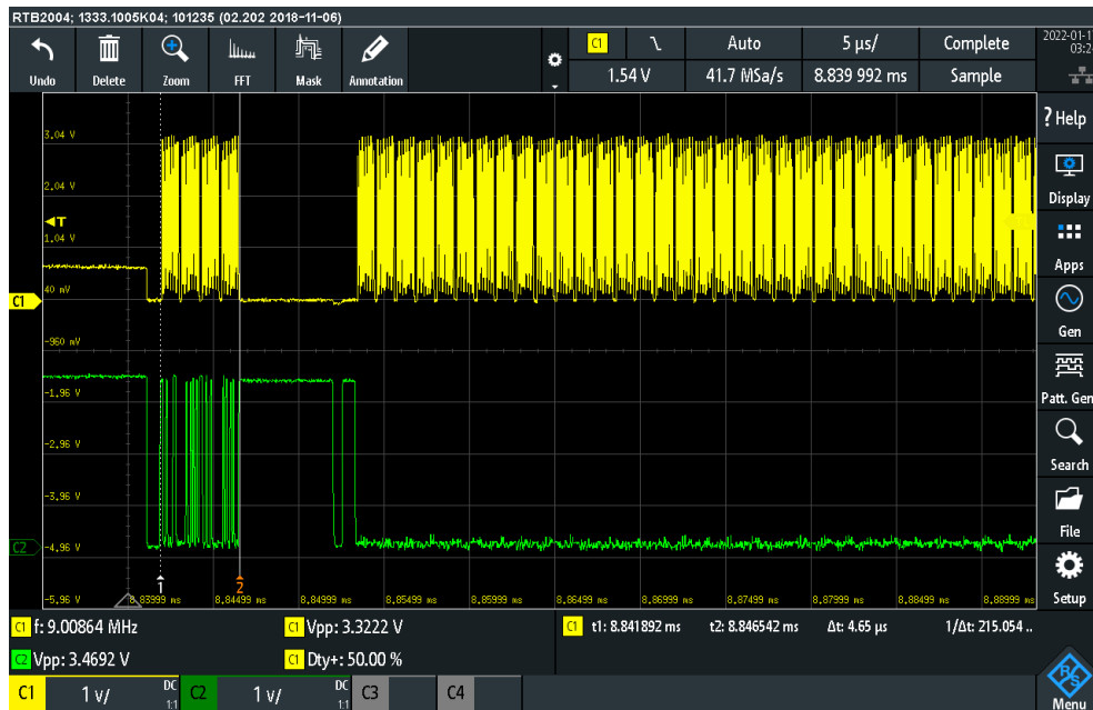
Figure 5.9: Closer view of the programming sequence and beginning of empty data. The spike that always occurs before empty data is also clearly visible.
