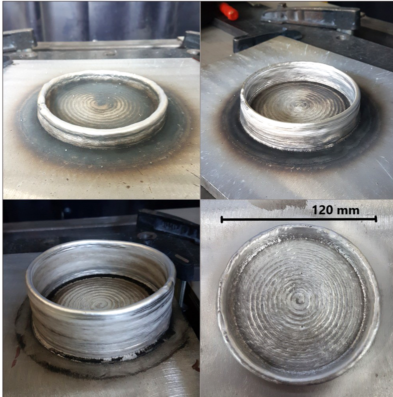
Fig. 8. Set-based: The structure was a cylindrical shape. The bottom layer was constructed in an outwards spiral, while the path for the wall was an upwards helix with a constant radius and a constant height increase.
