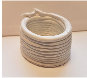
Fig. 12. Test results: The experimental work resulted in these small cups. It is evident that the width of the printed material, along with the height of the structure and the speed of the material deposition, are all important elements for the final result.
