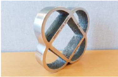
Fig. 10. Post processing: The Inconel 625 structure shown in fig. 6 after post processing. The opposing corners within each layer have merged together.
