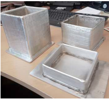
Fig. 4. Continuous build: Square-box structures with rounded corners and a smooth transition between layers.
