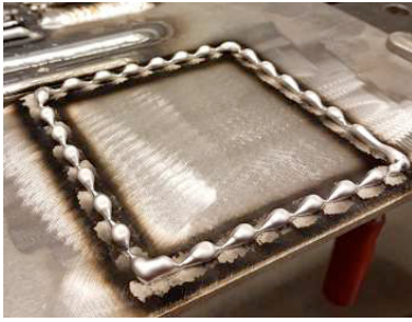
Fig. 9. Low heat input: Welding the first layers with a heat input that was too low made the deposited material clump together and not adhere properly to the base.
