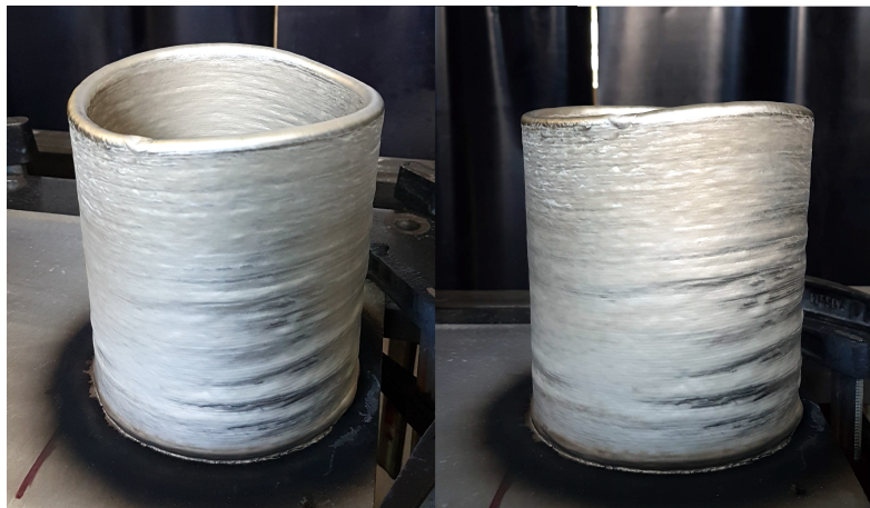
Figure 5.4: Set-based control: The resulting structure built using set-based control that allowed for a slack in the orientation of the welding gun of 6^\circ . The structure ended up having a saddle form, likely caused by the difference in gravitational pull on the deposited material, as the deviation in orientation of the welding gun was not symmetrically distributed.
