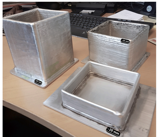
Fig. 5. Taller builds: After initial tests with square structures in aluminium, it was possible to build guide tall structures using material deposition.
