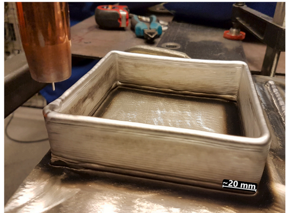
(b) Second, modified CMT box build with smoother walls and few distortions.
