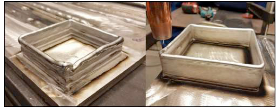
Fig. 2. Square-box: Smoother layer transitions, blunter corners and longer sides clearly improved the visual appearance of the structure.
