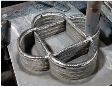
Fig. 7. Pulsed MIG: The final flower structure built in aluminium AA4043. This build has 65 layers, and some grinding were performed to reduce material accumulation in the intersections.
