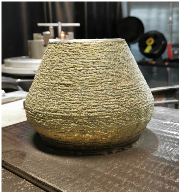
Figure 5.7: Vase with overhang: The vase structure with outwards and inwards tilting overhang, built by having the orientation of the tool approx. follow the tilt of the overhang.
