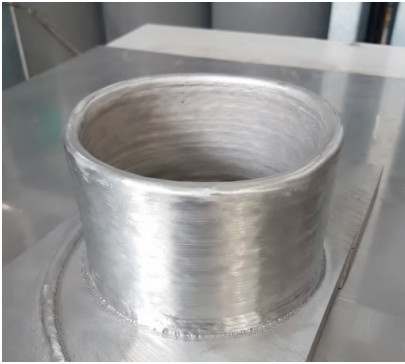
Fig. 4. Vertical welding gun: Cylindrical structure built with fixed, vertical orientation of the welding gun, with continuous height increase like that shown in Figure 2.
