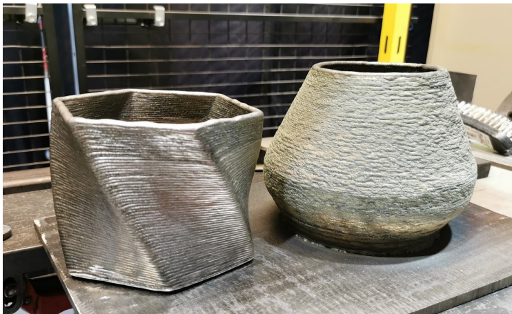
Figure 6.1: Overhangs: Two of the structures with overhangs built using the Ni–Cr–Mo alloy UTP759. For further details on these builds, see paper D [58].
