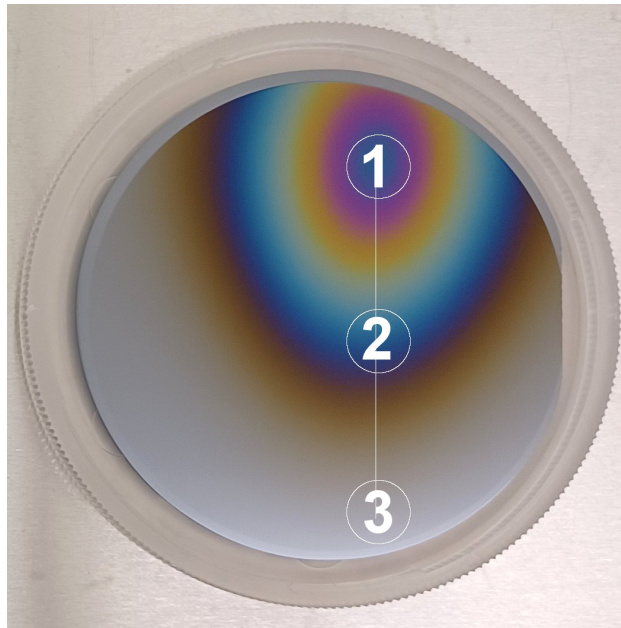
Figure 5.13: Photography of the wafer sample PTON550, and a schematic of the positions of measurement.
