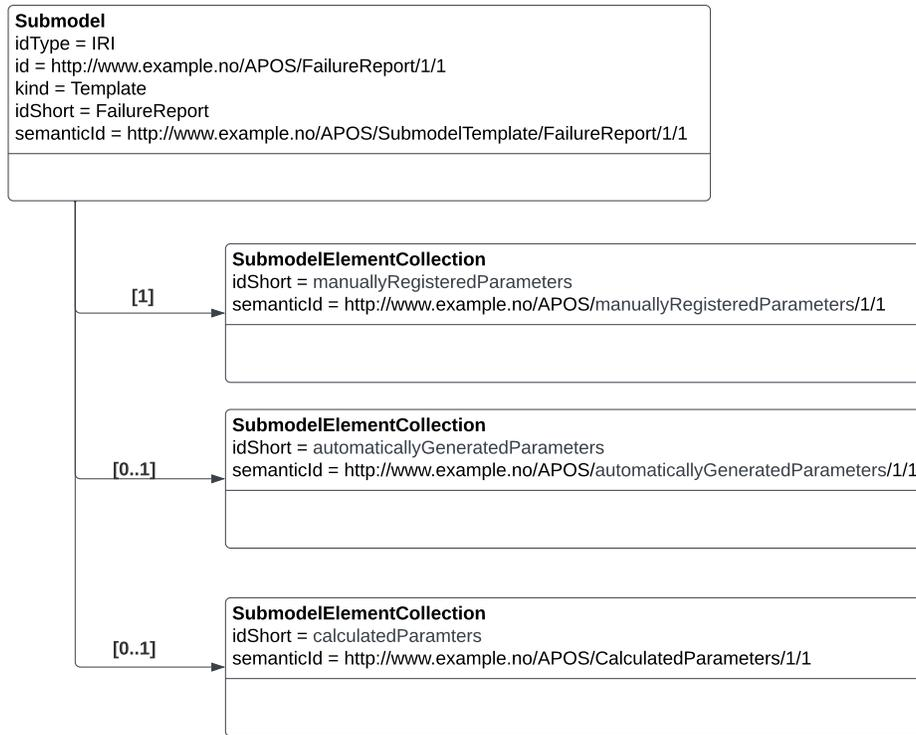
Figure 5.8: Submodel template for failure parameters
