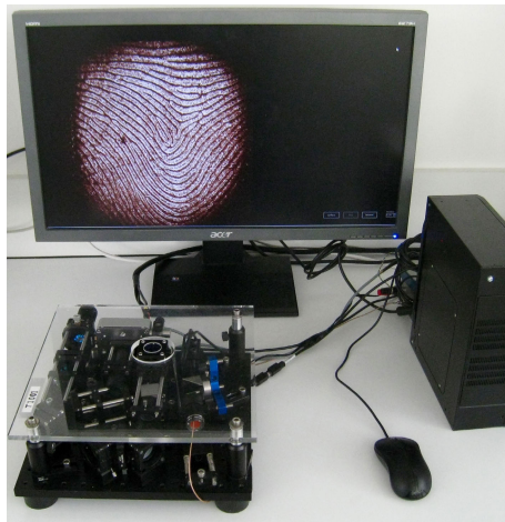
FIGURE 3. A complete compact and mobile FF-OCT fingerprint sensor system that includes the sensor, the microcomputer and the screen (which was not optimized in terms of size).
