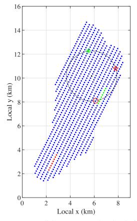
**Figure 1.** The PRMRA geometry. Not all the receivers are plotted in the figure for display purposes. The gather marked in red is used in the following example of beamforming. The gathers marked in green and red are used in the following examples of the NCC retrieval. The black circle and marks on it are used in the following study of events.
