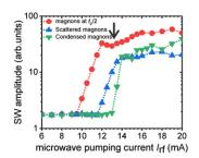
**Figure 5.** Amplitude of the parametrically generated magnons (red circles), the scattered magnons via (frequency-nonconserving) four magnon scattering processes (blue triangles) both under pumping and condensed magnons under relaxation (green triangles) as a function of the microwave current.
