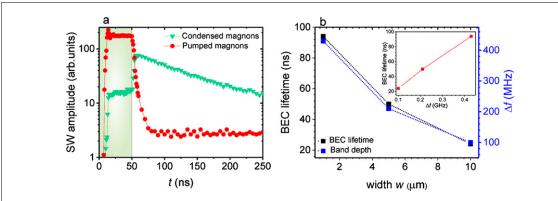
**Figure 4.** (a) Amplitude of the parametrically generated magnons (red circles) and condensed magnons at the band bottom (green triangles) as a function of time. The pumping pulse is distinguished via the green background color. (b) The lifetime of the BEC (black color) and band depth  $\Delta f$  with respect to the width of the conduits w. The inset shows the lifetime of the BEC with respect to the band depth  $\Delta f$ .
