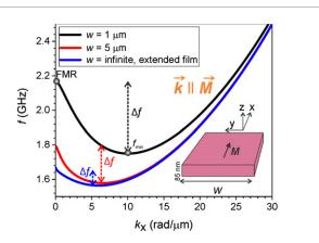
**Figure 1.** Dispersion relation of the lowest energy magnon band of a YIG thin film structure with a thickness of d = 85 nm and different degrees of confinement in one lateral direction.
