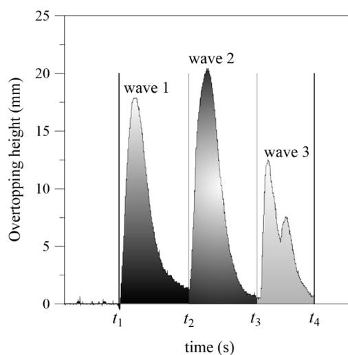
**Figure 6.** Overtopping height (mm) vs. time (s) plot for  $Q_{max}$  calculation considering the three maximum waves recorded in channel (CH) 11.
