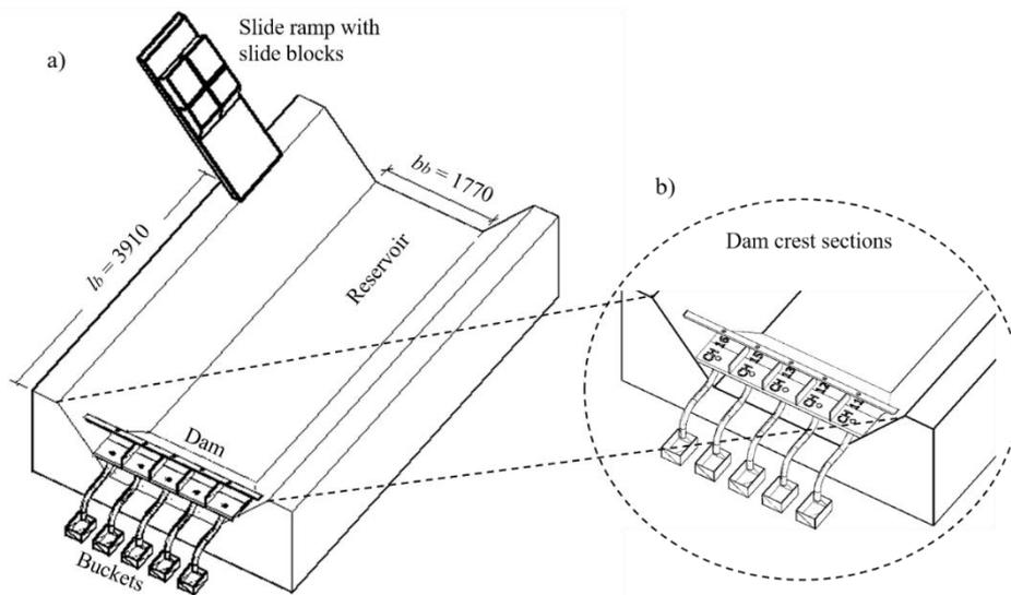
**Figure 2.** (a) Experimental setup with the main components; slide, reservoir, dam, and (b) ultrasonic sensors used for measuring the overtopping depth and buckets for collecting the overtopping water (all measurements are in mm).
