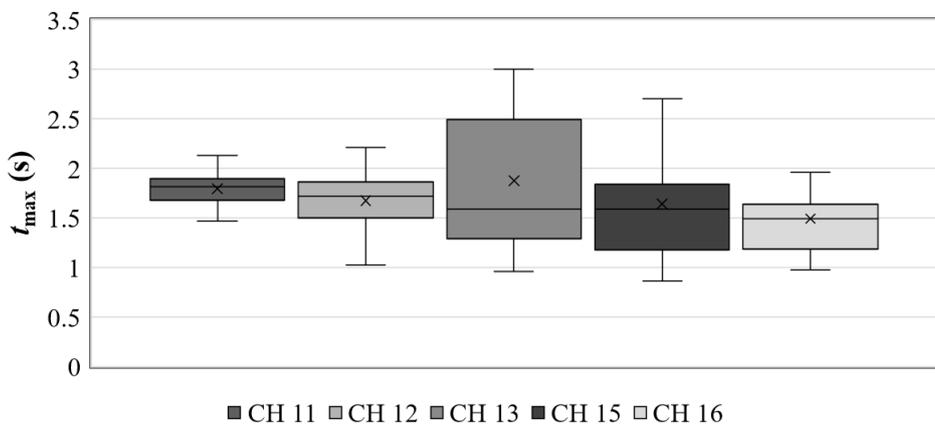
**Figure 12.** Box plot for the maximum overtopping duration for each channel along the dam crest.
