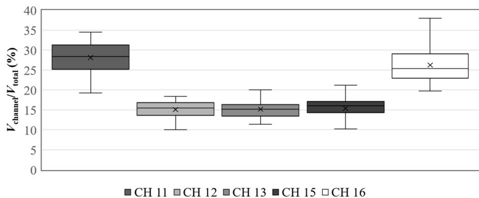
**Figure 5.** Overtopping volume distribution over the five dam crest sections (see Figure 2b for the position of sensors).
