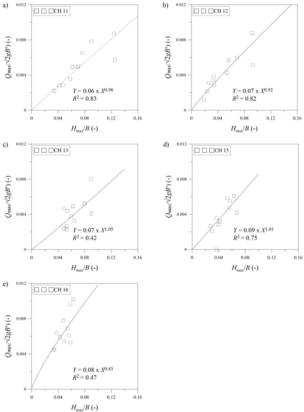
**Figure 7.** Plot between dimensionless measured maximum overtopping depth and calculated maximum discharge for CH 11, 12, 13, 15, and 16, respectively, for an upstream dam slope of 1 to 1.5 for  $C_d$  calibration.
