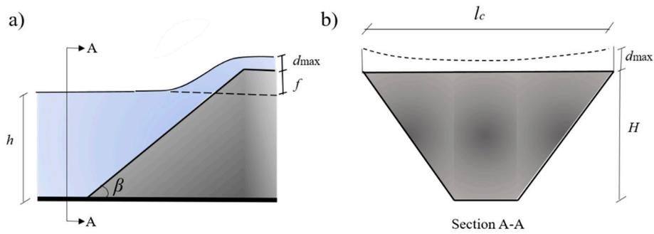
**Figure 3.** Definition sketch of the overtopping process with the input parameters for overtopping discharge over the dam crest: (a) side view, and (b) cross sectional view.
