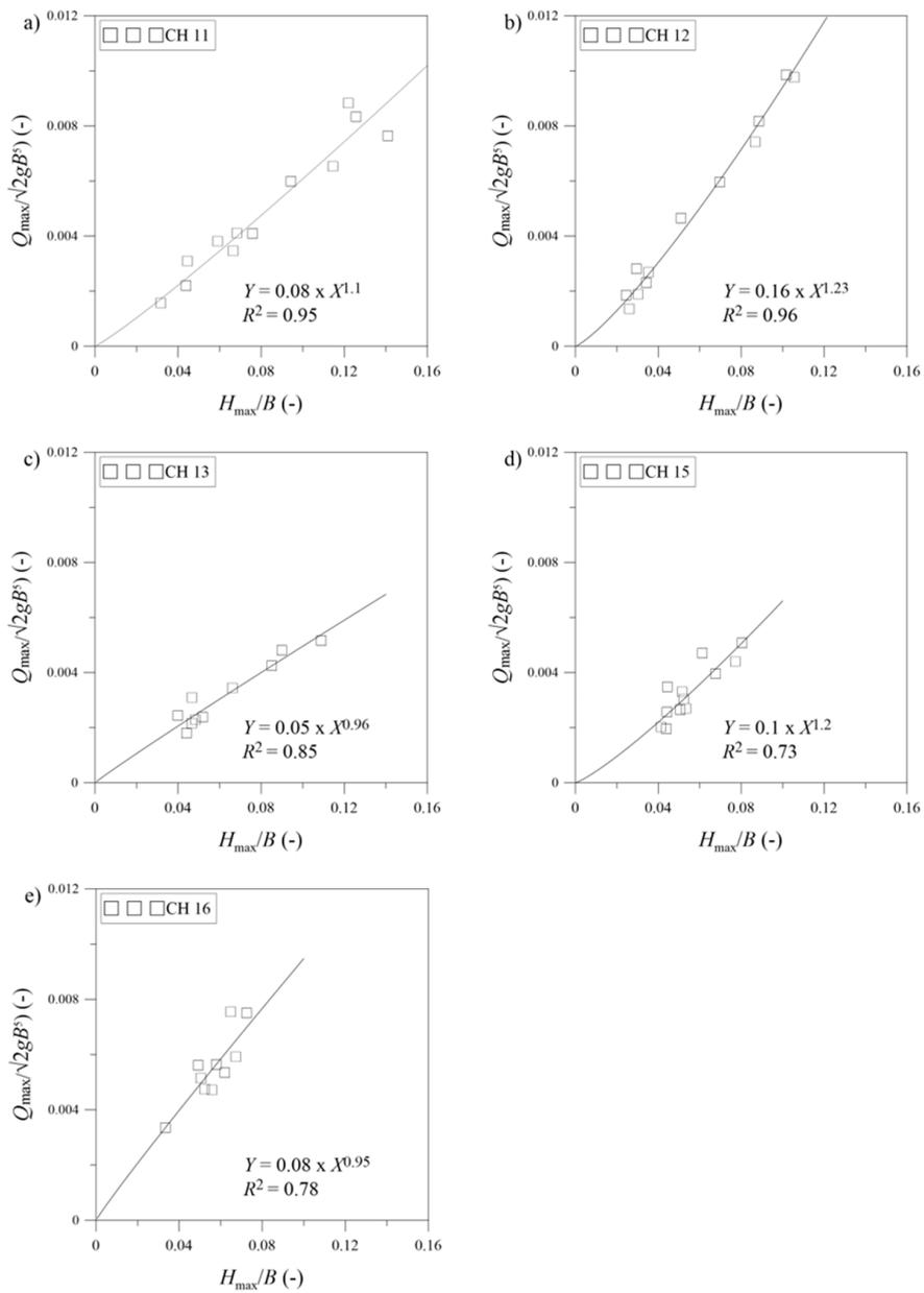
**Figure 8.** Plot between dimensionless measured maximum overtopping depth and calculated maximum discharge for channel 11, 12, 13, 15, and 16 for an upstream dam slope of 1 to 2.25 for  $C_d$  calibration.
