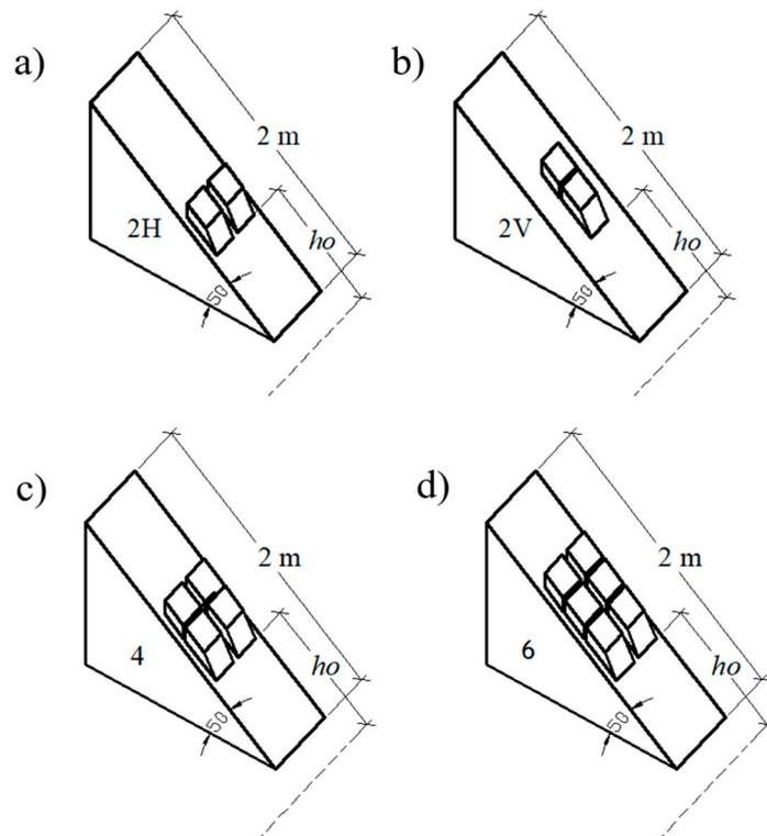
**Figure 4.** Arrangement of block configurations used in the tests with  $h_0$  parallel to the ramp slope and measured from the still water level: (a) 2H; (b) 2V; (c) 4 blocks and (d) 6 blocks arrangement.
