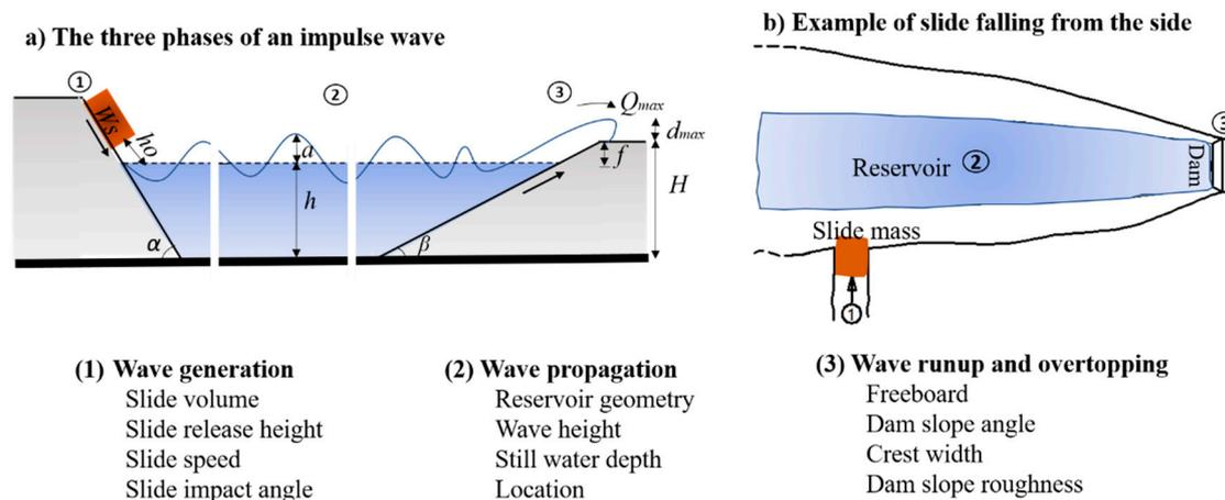
**Figure 1.** The three phases of landslide generated waves with the governing parameters: (1) slide impact with wave generation; (2) wave propagation; and (3) wave run up and overtopping of a dam. (a) A section showing the three phases based on Heller et al. [14]; (b) an example plan view of a reservoir.
