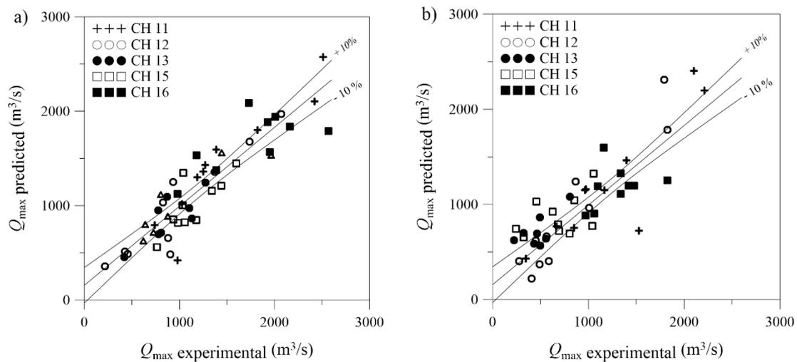
**Figure 10.** Comparison of calculated and predicted maximum discharge over the dam crest for upstream dam slopes; (a) 1 to 1.5 ( $R^2 = 0.82$ ) and (b) 1 to 2.25 ( $R^2 = 0.72$ ) (full scale), with  $\pm 10\%$  deviation.
