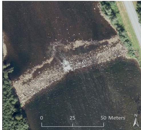
Figure 2 Weir no. 11 in River Nea. Total width of the weir is 105 m and the drop in water surface from upstream to downstream is 0.98 m on a flow of 2 m 3 /s.
