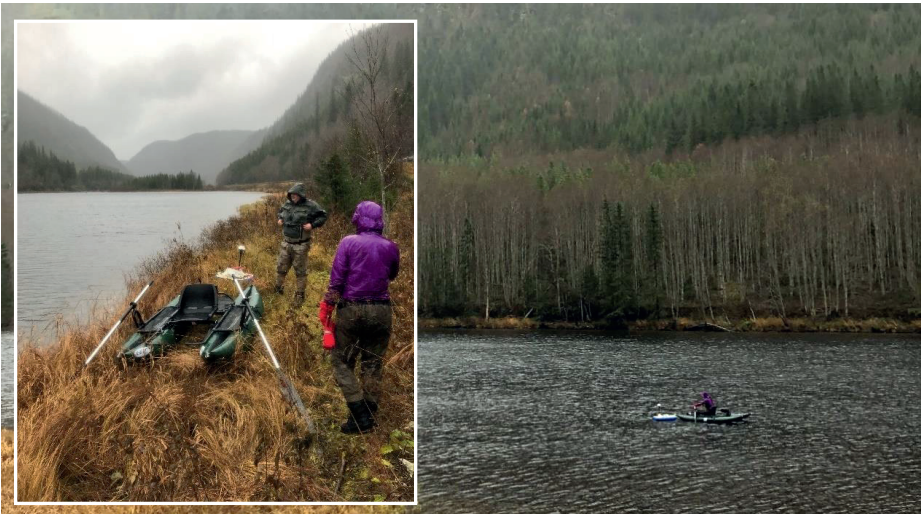
Figure 6. Calibration data on depths and velocities in River Nea was measured using a catamaran-type boat carrying an M9 RiverSurveyor from SonTek. Photo: Håkon Sundt
