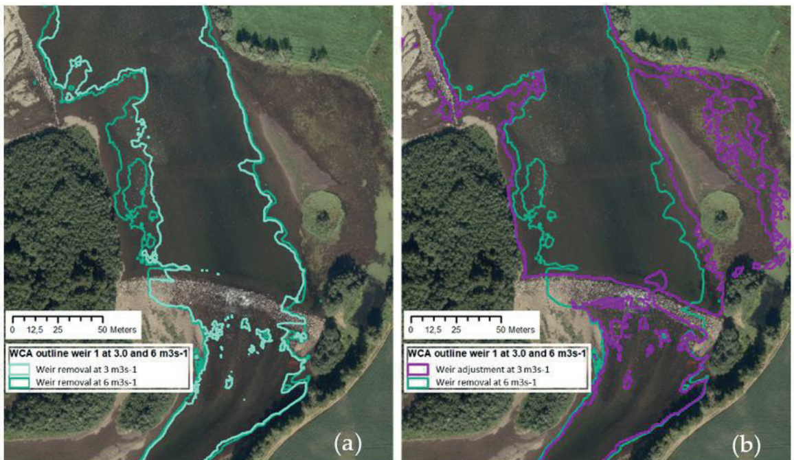
Figure 9. Example of the effect of weir adjustment and removal on the water-covered area for weir no. 1 at flows 3 and 6 \text{ m}^3/\text{s} . (a) WCA outline for full weir removal simulated at flows of 3 \text{ m}^3/\text{s} (light green) and 6 \text{ m}^3/\text{s} (dark green). (b) WCA outline for weir adjustment at 3 \text{ m}^3/\text{s} (purple) and weir removal at 6 \text{ m}^3/\text{s} (dark green). As shown in (b), doubling the flow to 6 \text{ m}^3/\text{s} with weir removal compensates for a large proportion of the WCA for weir adjustment at a flow of 3 \text{ m}^3/\text{s} .
