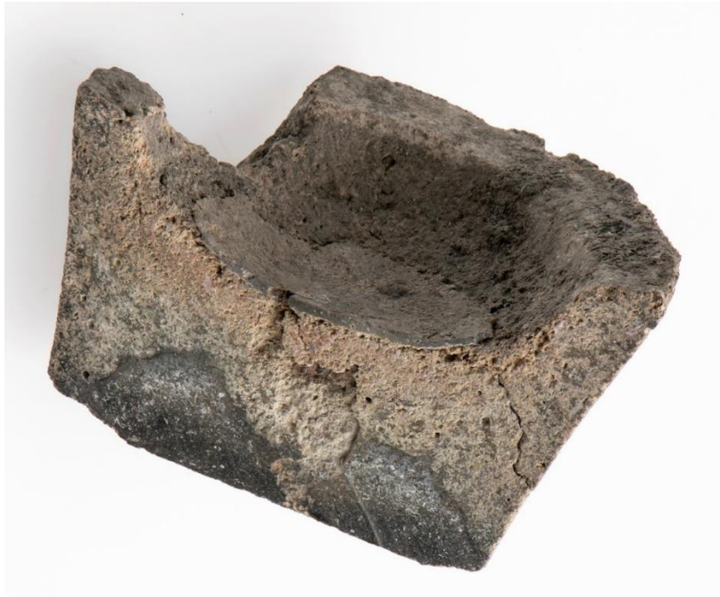
Figure 4. Cross-section of cupel N124860. Upper rim diameter 35 mm, height 23 mm. Note the fine-grained surface layer (i.e. the facing) at the bottom of the bowl and the two dark areas at the bottom of the cupel where lead oxide has filled both cavities between the bone-ash particles and the canals in the bone-ash, in contrast to just in the canals in the bone-ash particles higher up. Photograph: Åge Hojem, NTNU University Museum.
