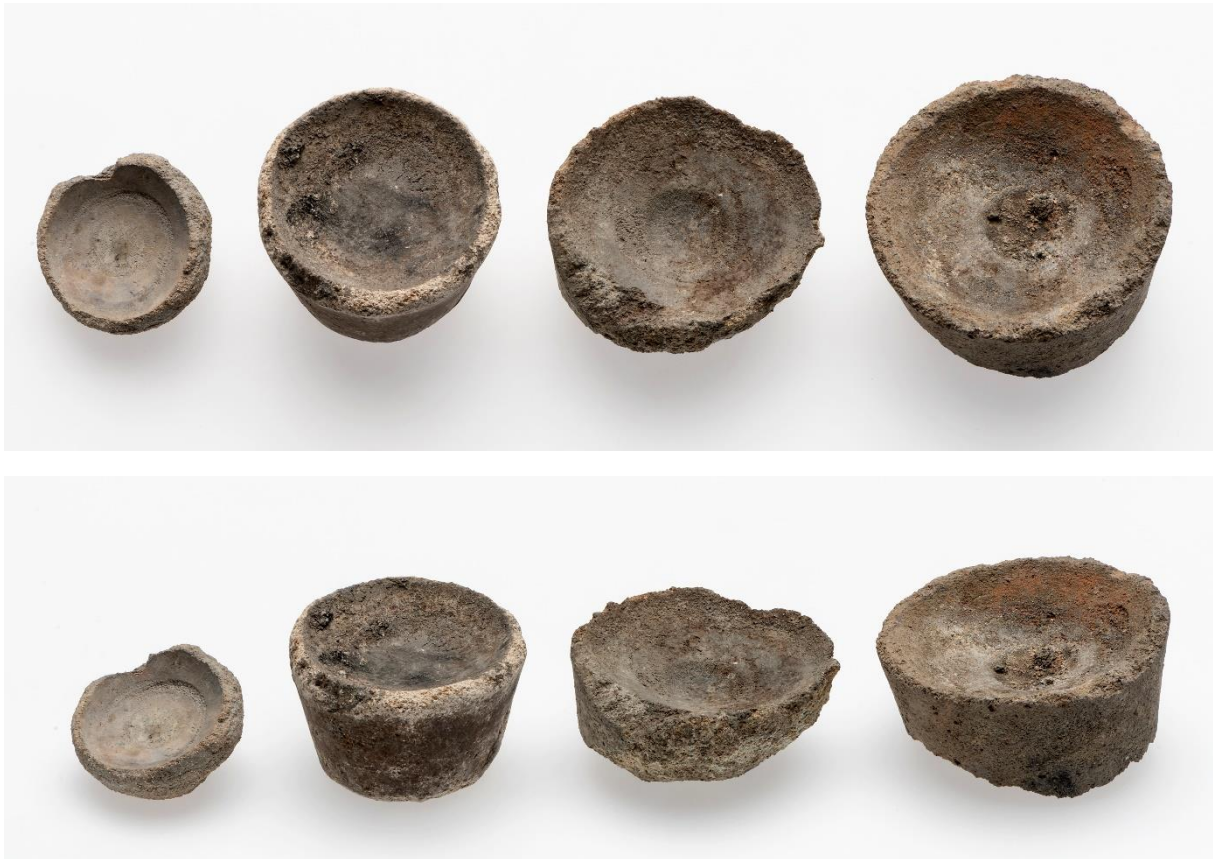
Figure 3. Four bone-ash cupels viewed from two angles. From left to right, they have an outer rim diameter of 30 mm (N125123), 35 mm (N122514), 40 mm (N124858), and 45 mm (N124857), respectively. Note the depression at the bottom of the largest cupels, N124857 and N124858. Photograph: Åge Hojem, NTNU University Museum.
