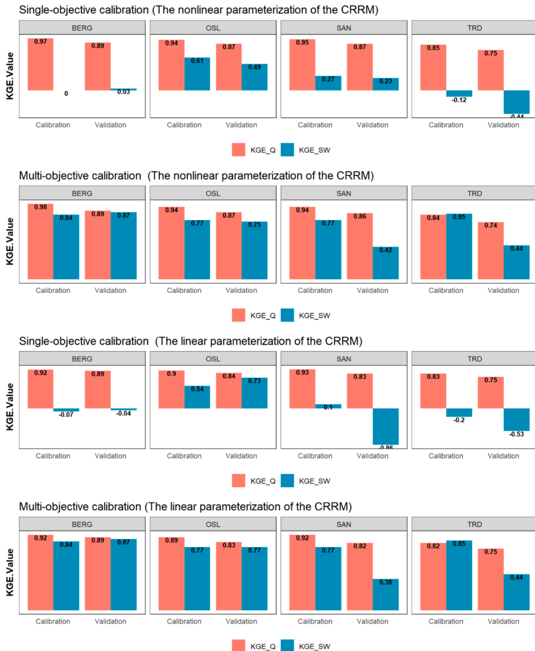
Fig. 2. Comparison between the two calibration schemes and the two parameterizations of the CRRM at Thin2 roofs.
