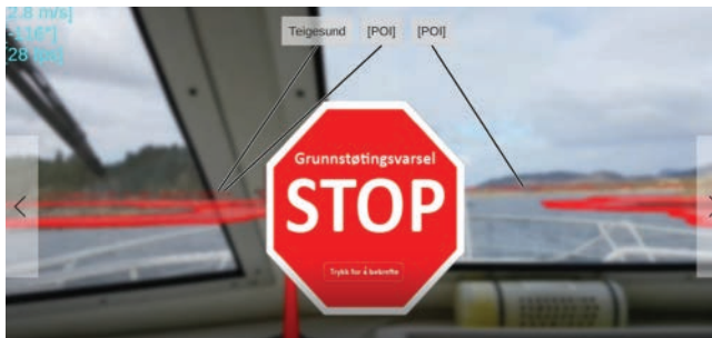
FIGURE 8.6 Screen dump from the Galaxy test phone. The grounding alarm has been triggered with both an aural and a visible alarm. (Photo courtesy of the author.)
