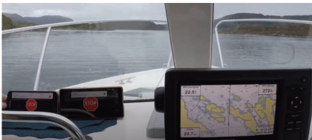
FIGURE 8.9 Tests in October 2019. To the left two tested smart phones where the grounding alarm has just been triggered. To the right the chart plotter shows speed position, heading and distance to the triggering depth curve. (Photo courtesy of Harald Notøy and Leidulf Garshol.)
