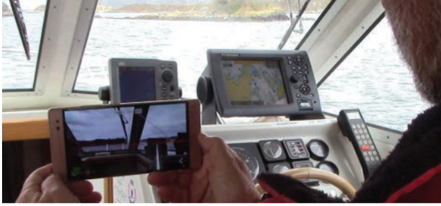
FIGURE 8.4 The test application on the smartphone (Lenovo Phab 2 Pro) during the pilot test. To the right, the boat’s reference stationary chart plotter. (Photo courtesy of the author.)
