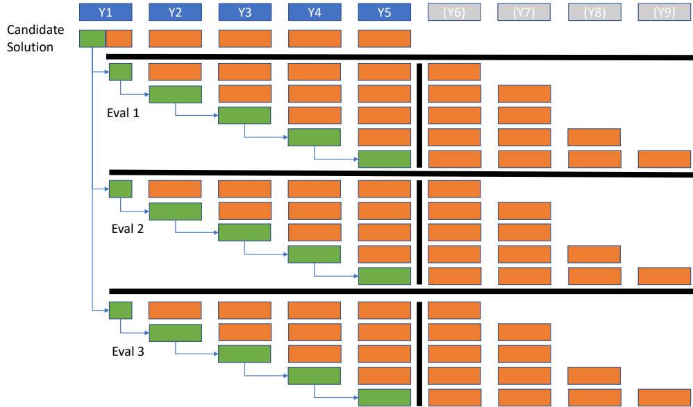
Figure 7.4: Schematic overview of the evaluation of a candidate solution to the first-stage variables of the first primary period.
