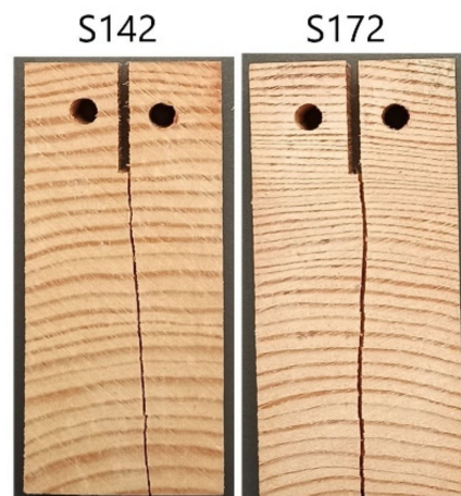
Figure 18. Shape of the fractures in samples S142 (Group 1) and S172 (Group 2).
