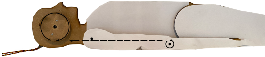
Figure 3.8: Elbow joint actuation system
