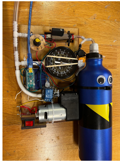
(b) The complete pressure control rig
