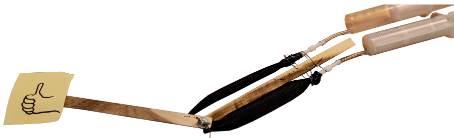
Figure 3.2: First prototype using McKibben muscles
