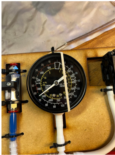
(a) Vacuum achieved by the prototype rig
