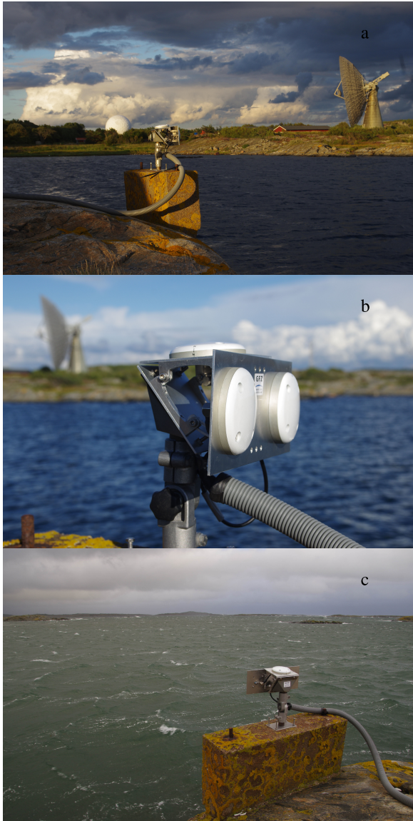
Fig. 5. Eastward view of the GFZ GNSS-R station at (a) OSO, (b) zenith looking, RHCP, and side looking, RHCP and LHCP, antennas, and (c) sea targeted at the antenna boresight.
