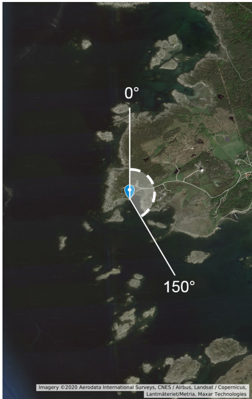
Fig. 10. GNSS-R station location and the wind azimuth range condition (0°–150°) in the analysis.
