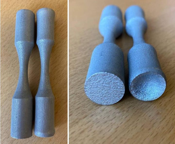
Figure 2: Comparison of solid and shelled geometries subsequent to HIP – shrinkage of shelled geometry is visible.
