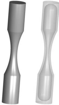
Figure 1: Fatigue hourglass specimen geometry shown with solid view (left) and shelled geometry and internal cavity visible in the transparent view – central cavity is 3 mm wide in 6 mm gauge diameter at narrowest section.
