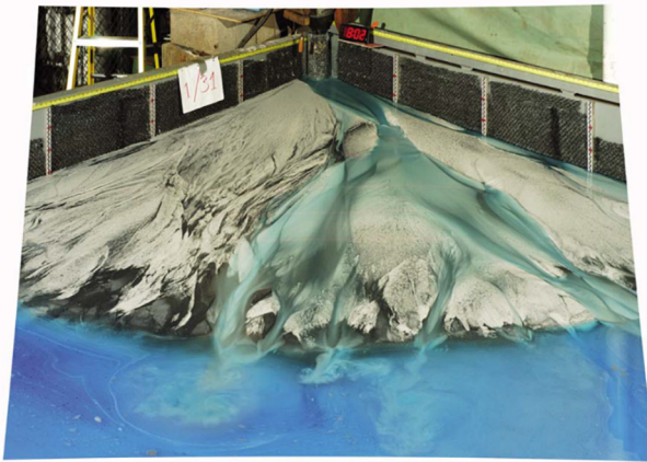
Fig. 4. Example of an experiment using an analogue-landscape modelling approach (Sheets et al., 2002; Ganti et al., 2011). (a) Schematic of the experimental set up. (b) Photography of the delta after 11 h of experimental run time. From Ganti et al. (2011).
