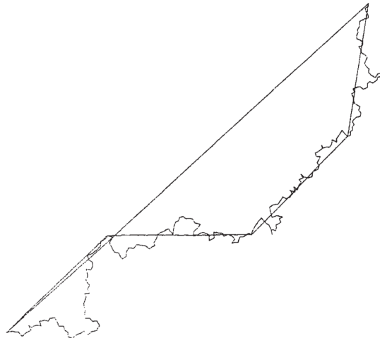
Figure 2.6: Fractal polyline with 2, 5, and 257 points created by multiple iterations of midpoint displacement [15].
