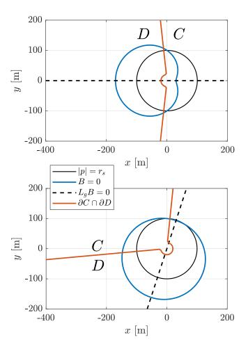
Fig. 1. Illustration of flow set *C* and jump set *D*, projected onto  $\mathbb{R}^2$ , for  $q_0 = 0$  (top), and  $q_0 = q_1 = 1$  (bottom). Fixed  $z = [1 \ 0]^\top$ , i.e. vehicle traveling from left to right. Parameters; v = 5,  $r_s = 100$ ,  $\epsilon = 20$ ,  $k_1 = \frac{\pi}{3}$ ,  $t_1 = 7.16$ ,  $t_0 = t_1(1 + \sin(k_1))$  and  $\delta = \frac{\mu}{4}$ .
