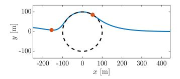
Fig. 2. Trajectory of p in the  $\mathbb{R}^2$ -plane. The vehicle is traveling from left to right. The red dots mark where the CBF becomes active and inactive. Boundary of  $\mathcal{K}_u$  shown in dotted black lines, corresponding to  $|p| = r_s$ .
