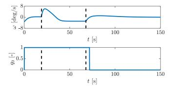
Fig. 3.  $\omega$  (top) and  $q_0$  (bottom) corresponding to the trajectory in Figure 2. The dashed horizontal lines indicate when the CBF becomes active and inactive.
