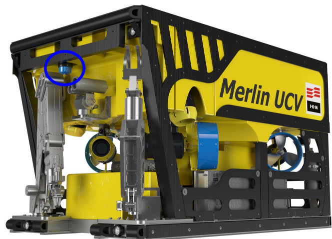
Fig. 1. The Merlin UCV. The sonar position is highlighted in blue.
