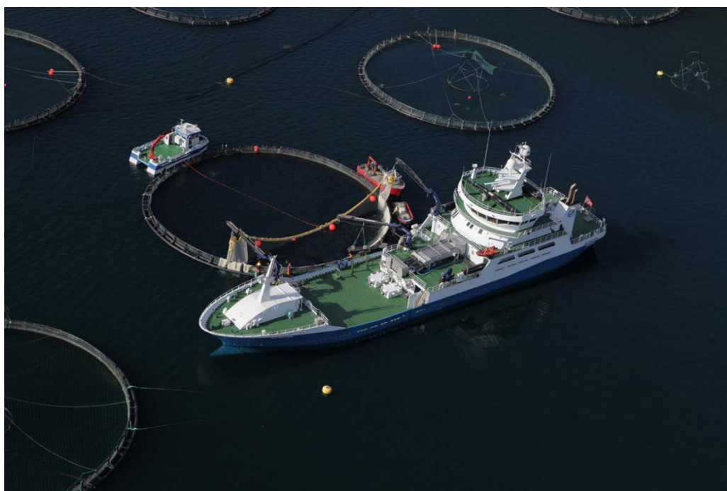
Figure 2 A fish crowding and sorting operation. (Picture reproduced with permission from Rostein AS.)
