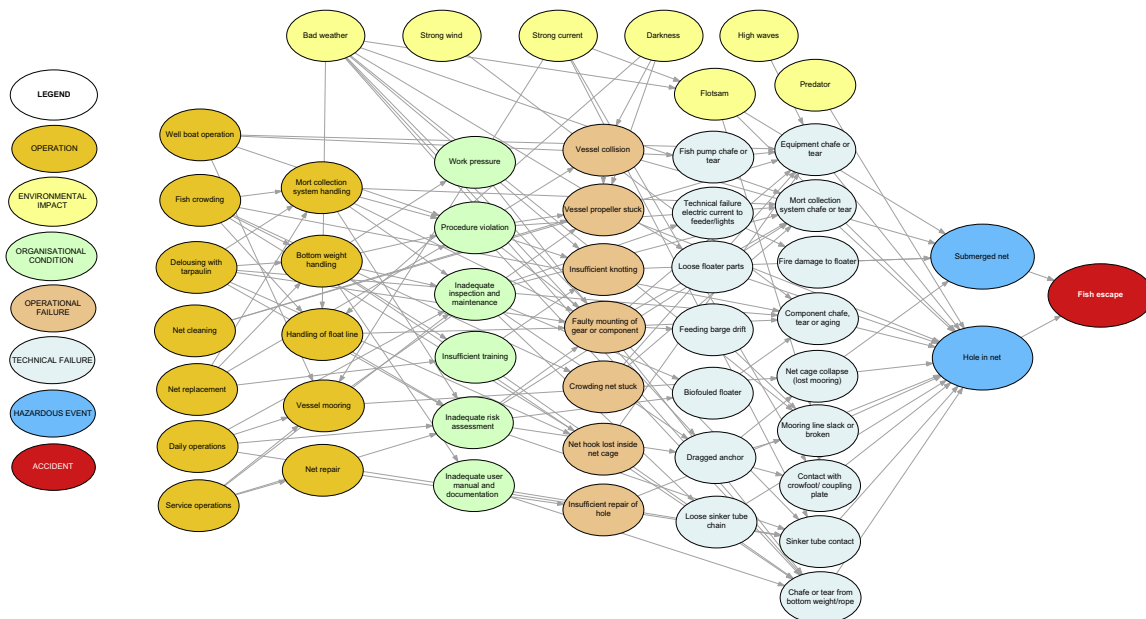
Fig. 2. Graphical illustration (BN) of causal chains for escape of farmed fish caused by a hole in the net or a submerged net.
