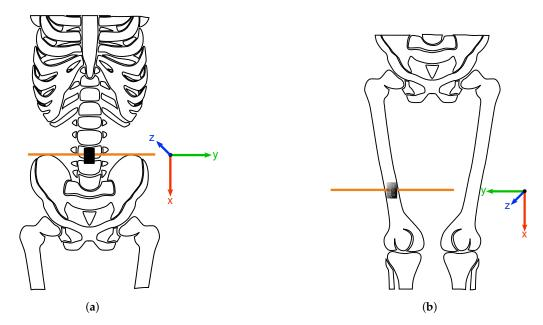
**Figure 1.** This figure shows the two sensor positions (highlighted with orange lines) used for our dataset. (**a**) The lower back sensor is positioned at approximately the 3rd lumbar vertebra. The z-axis of the coordinate system points forward. (**b**) The thigh sensor is positioned approximately 10 cm above the upper kneecap. The z-axis points backward.
