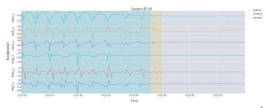
**Figure 3.** This figure shows ten seconds (x-axis) of the acceleration signals (on the y-axis and in  $m/s^2$ ) of all three axes of the back and thigh accelerometers. We focus on the subject with subject ID 28. The background is shaded according to the activity label, in this case walking (green), shuffling (yellow), and standing (gray).
