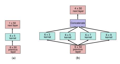
Figure 4. This figure illustrates a single layer in a standard CNN (a) and a multi-resolution CNN (b).
