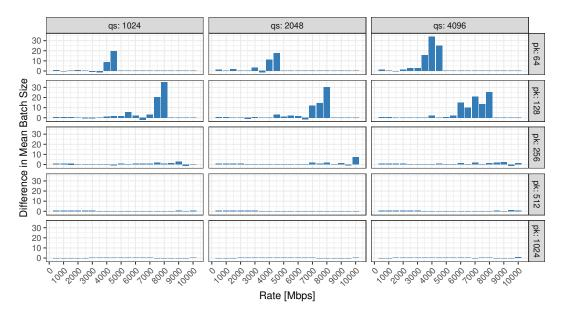
Fig. 9. Difference in mean batch sizes obtained via model and measurements given different packet (pk) and queue sizes (qs). Maximum batch size  $\beta = 256$  and mixed traffic. Values greater than 0 correspond to the mean batch size in the measurements being larger than the one returned by the model.
