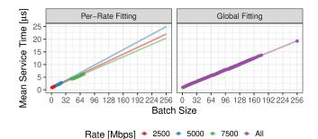
Fig. 5. Size-dependent batch service times. Points indicate mean values from measurements, lines denote linear fits. Cross-connect scenario with  $\beta = 256$ , L = 4096, and 64 B packets.
