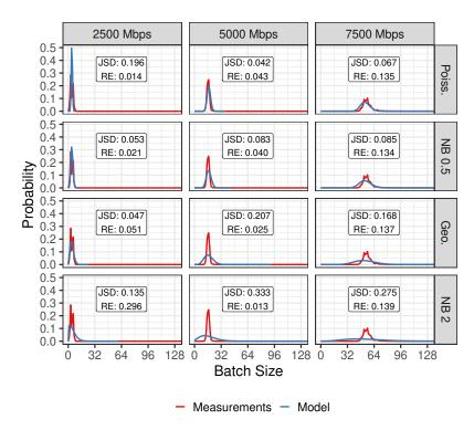
Fig. 7. Batch size distributions for different rates and arrival processes. Cross-connect scenario with  $\beta$  = 256, L = 4096, and 64 B packets.
