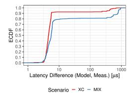
Fig. 12. Distribution of the latency difference between measurements and the model. All scenarios are included, i.e., queue size  $L \in \{1024, 2048, 4096\}$ , maximum batch size  $\beta \in \{64, 256, 512, 1024\}$ , and packet size  $\in \{64, 128, 256, 512, 1024\}$  B.
