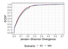
Fig. 10. Distribution of the Jensen-Shannon divergence regarding the batch size distributions obtained from measurements and via the model. All scenarios are included, i.e., queue size  $L \in \{1024, 2048, 4096\}$ , maximum batch size  $\beta \in \{64, 256, 512, 1024\}$ , packet size  $\in \{64, 128, 256, 512, 1024\}$  B, and applied rate  $\in \{500, 1000, \ldots, 10000\}$  Mbps.
