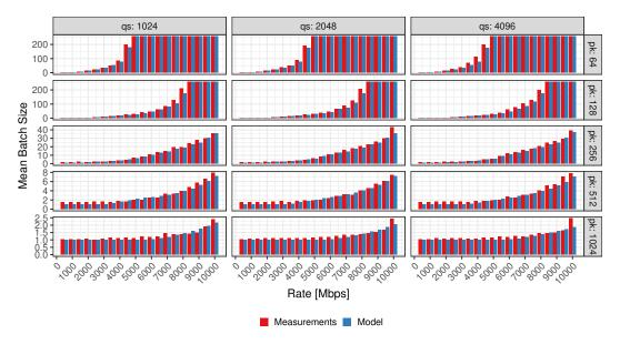
Fig. 8. Average batch size obtained via model and measurements given different packet (pk) and queue sizes (qs). Maximum batch size  $\beta = 256$  and mixed traffic.
