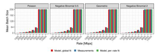
Fig. 6. Mean batch sizes for different rates, arrival processes, and fitting strategies. Cross-connect scenario with  $\beta$  = 256, *L* = 4096, and 64 B packets.
