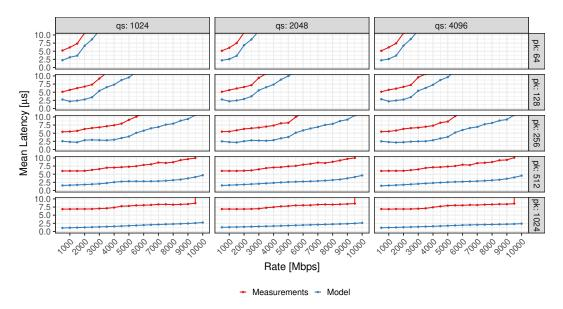
Fig. 11. Mean latency measured in the technical system and reported by the model under different packet (pk) and queue sizes (qs). Maximum batch size  $\beta = 256$  and mixed traffic.
