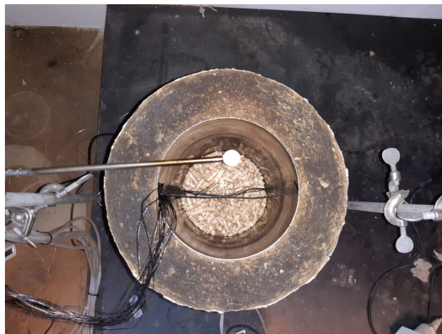
Figure 17: Photo of the bidirectional probe, thermocouple-ladder with regards to the pipe and sample.
