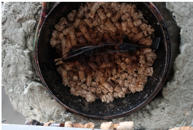
Figure 32: Picture of the underside of the steel cylinder containing the sample. The picture is taken after a test, and the black burned pellets is at height 2 cm.
