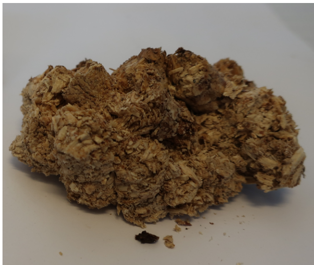
Figure 33: Picture of a piece of pellets after a test where bridging occurred.
