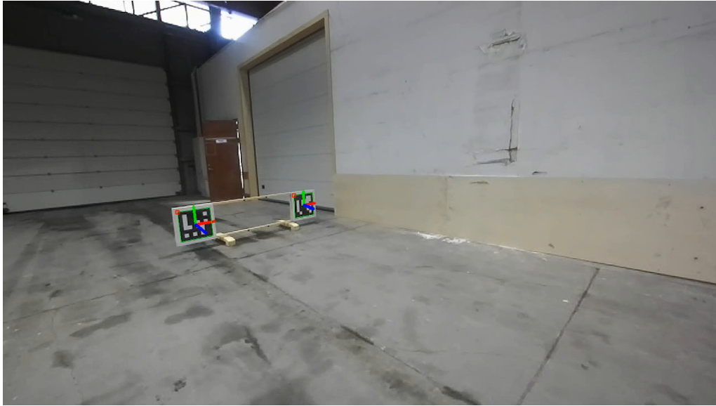
Figure 3.9: Detection of two 0.412m \times 0.412m markers with the aruco detection algorithm, with 1280 \times 720 resolution. Link to recording: https://www.youtube.com/watch?v=EGs43mpN0DE .
