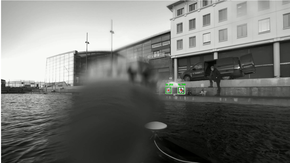
Figure 4.11: Marker detections with water droplet on the camera lens. Here marker ID 227, which is used to estimate the USV position is concealed by a water droplet.
