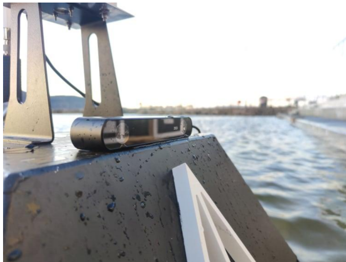
Figure 3.5: The ZED2i camera mounted on the Otter USV.
