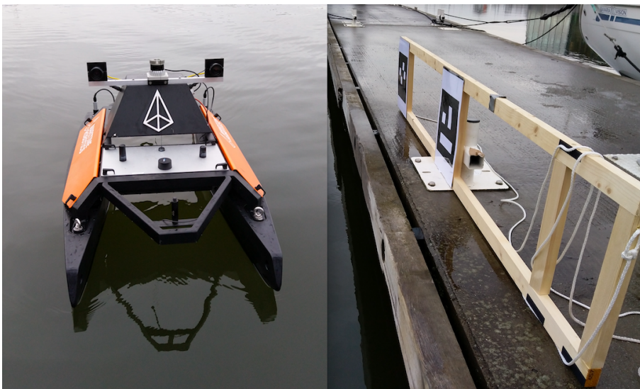
Figure 2.4: Illustration of Ø. Volden experiment with a Otter USV and fiducial markers on the pier. Image courtesy to Ø. Volden [16].
