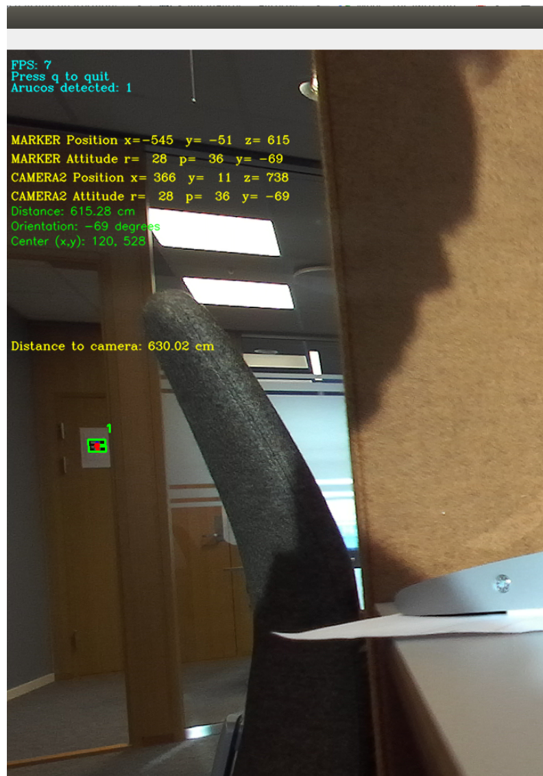
Figure 3.8: Detection of a 10\text{cm} \times 10\text{cm} aruco marker from a distance of 6.30 m. Calculation of the camera orientation to the marker is also displayed in the image (image screenshot by the computer screen).
