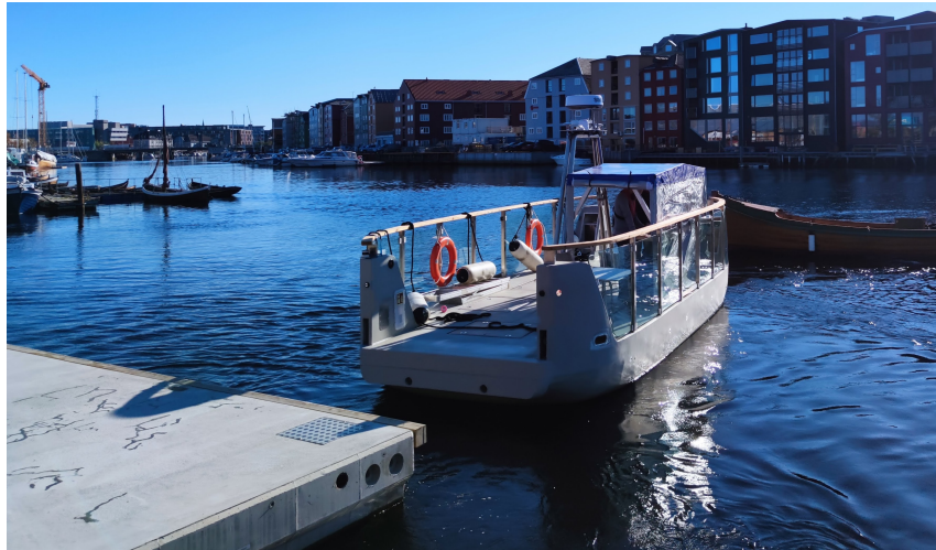
Figure 2.3: milliAmpere2 in the docking phase. Developed by NTNU as a research project for autonomous system. The overall goal of the project is to develop intelligent solutions to bring passengers from place a to a place b.
