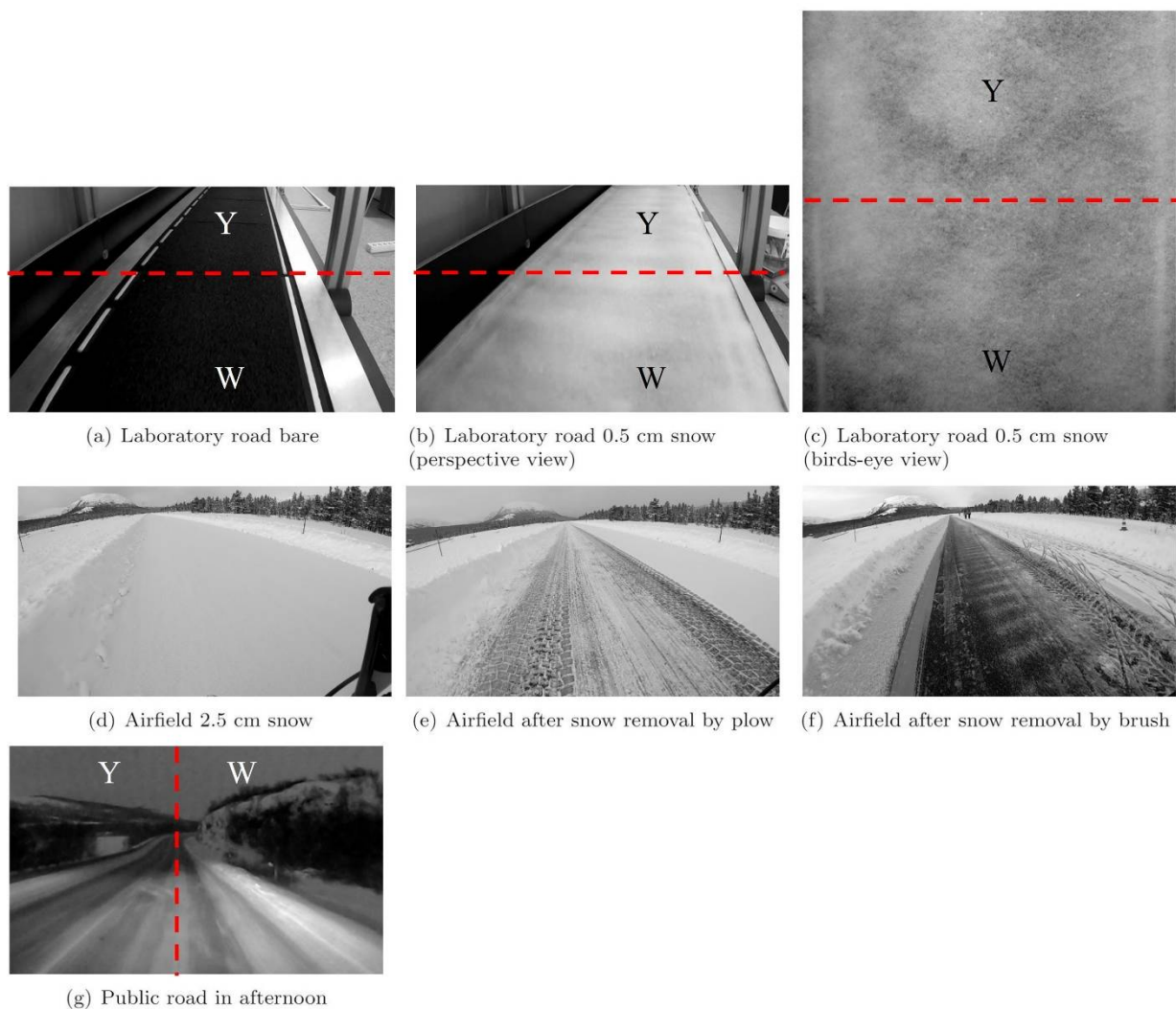
Figure 9. Grayscale representation of the seven different cases. The red lines separate the parts of the images containing white (W) and yellow (Y) markings, respectively.
