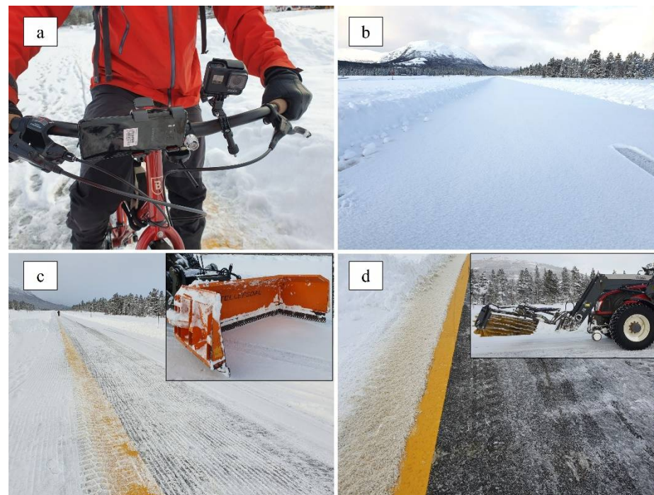
Figure 8. (a) Video capture set-up for airfield scenario, (b) 2.5 cm snow coverage on test track, (c) Test track after snow removal by ribbed snowplow, and (d) Test track after snow removal by brush.
