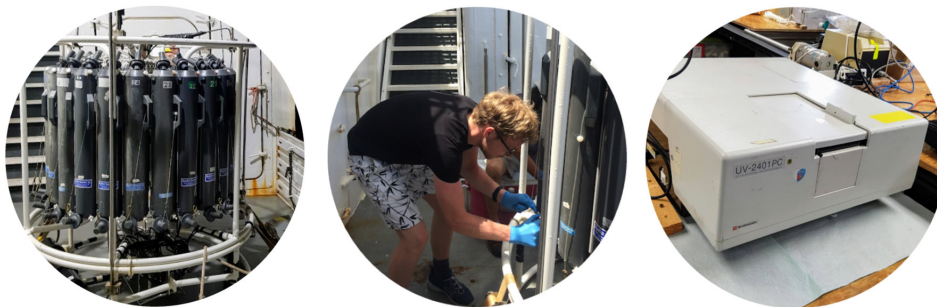
Figure 4.4.: Tools and methods used during sampling. The image on the left depicts a rosette station with Niskin bottles for CTD measurements, while the center image shows the collection of water from the rosette station. the rightmost image shows the spectrometer which was used to analyze the absorption properties of the collected water samples in-situ. Center photo shows me collecting data during the 2019 Cruise.
