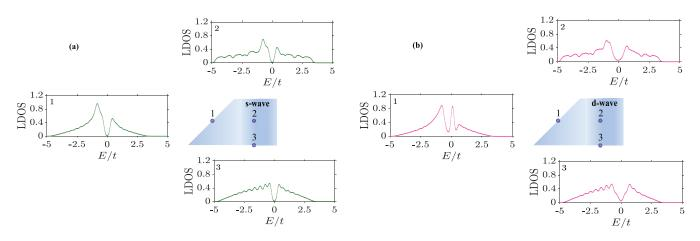
FIG. 2. Local density of states (LDOS) for different points of an *s*-wave superconductor (a) and a *d*-wave superconductor (b), showing the presence of midgap states on the diagonal edge of the *d*-wave superconductor. In both cases the size of the structure is  $L_{xS} = 34$  and  $L_{yS} = 30$ . For the *s*-wave results we have taken U/t = 2 and V = 0, while for the *d*-wave results we have taken U = 0 and V/t = -1. In both cases we have set the chemical potential  $\mu_S = 0.7t$ .
