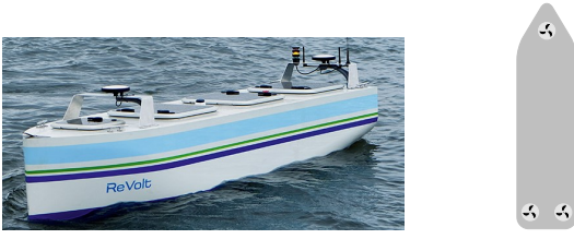
Figure 2: The Revolt test platform is a 1 : 20 scale model of an autonomous concept vessel with two fully rotatable azimuth thrusters in the stern and one fully rotatable azimuth thruster in the bow.
