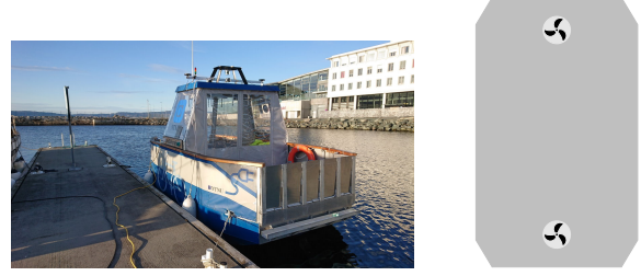
Figure 3: The MilliAmpere test platform has two fully rotatable azimuth thrusters along the centerline of the vessel.
