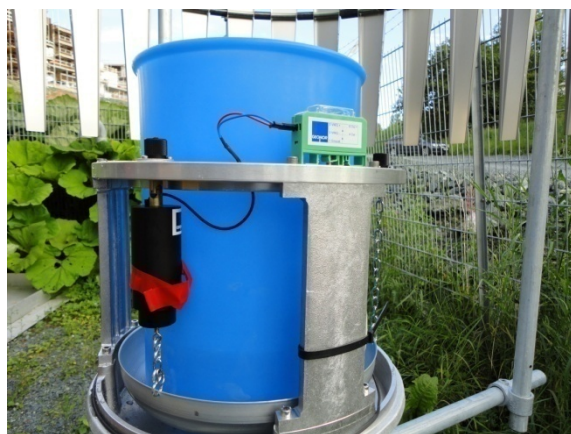
Figure 70: Geonor T200 – B gauge opened
