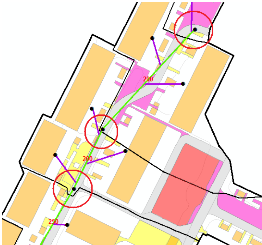
Figure 10: Connected manholes located at the downstream border of its respectable sub catchment
