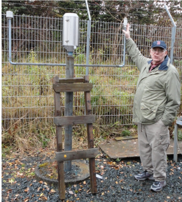
Figure 72: Associate Professor Sveinn T. Thorolfsson explains about the Lambrecht gauge
