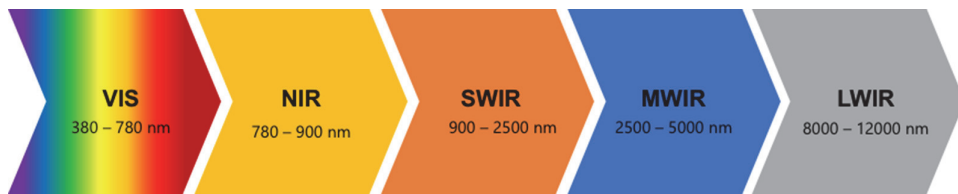
Figure 5.2 Electromagnetic spectrum, from left to right: VIS (380–780 nm), NIR (780–900 nm), SWIR (900–2500 nm), mid-wave infrared (MIR: 2500–5000 nm), and long-wave infrared (LWIR: 8000–12,000 nm). The wavelength range 5000–8000 nm is defined as a stop band due to very high absorption and is therefore omitted.
