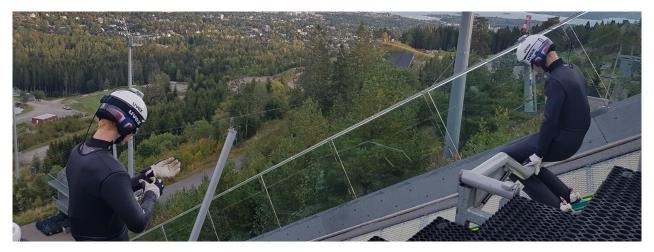
Figure 2. Ski jumpers with the dGNSS antennae mounted on their helmets and the receivers in backpacks that were carried under the ski jumping suit.
