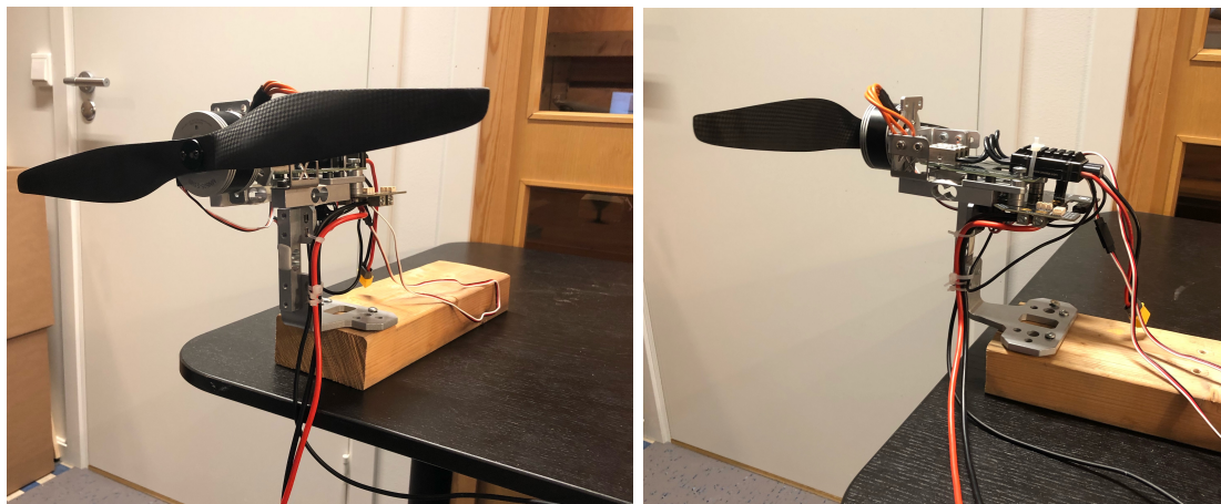
Figure 4-4: Experimental setup used for measurements of the propeller constants.
