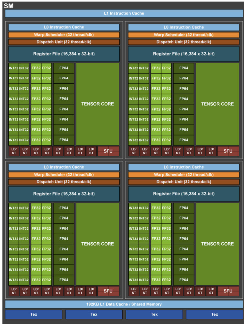
Figure 2.3: The A100 SM architecture From https://developer.nvidia.com/blog/nvidia-ampere-architecture-in-depth/ Figure is used with permission from NVIDIA.
