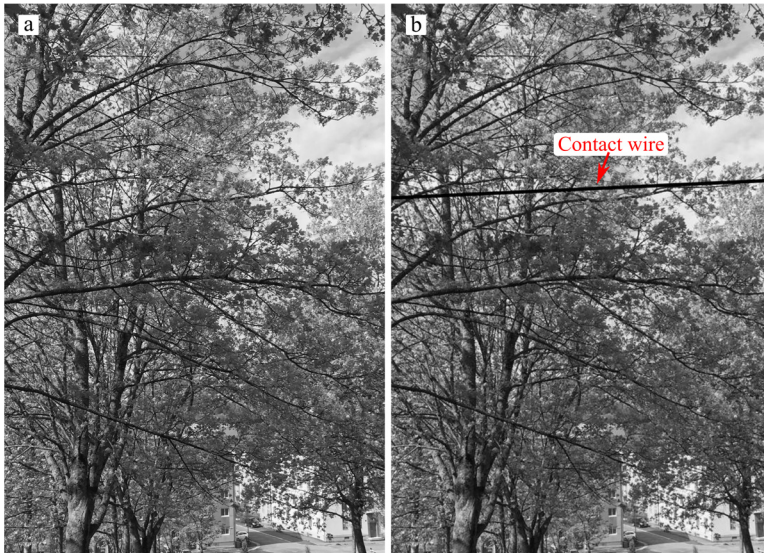
Fig. 2.12. Noisy background image. (a) Original image. (b) A black line is used as a contact wire in front of the noisy background. Photo: Tengjiao Jiang/NTNU.
