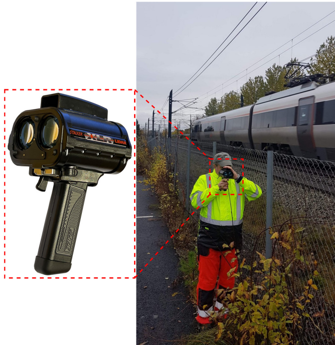
Fig. 4.7. Measuring method of train speeds. Photography: Tengjiao Jiang/NTNU.
