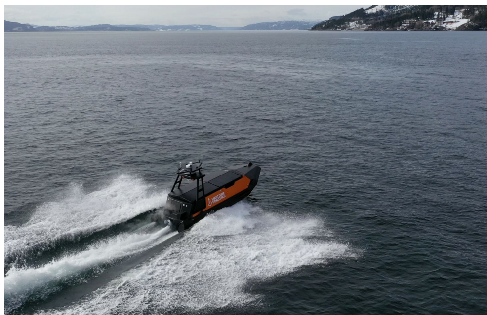
Figure 2. The Maritime Robotics Mariner USV (dimensions 5.95 \times 2.05 \times 2.00 m and weight 1900 kg) [3].
