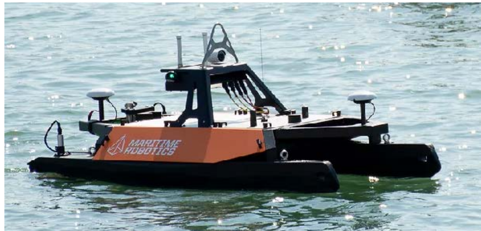
Figure 1. The Maritime Robotics Otter Pro USV (dimensions 2.00 \times 1.07 \times 0.82 m and weight 65 kg) [3].
