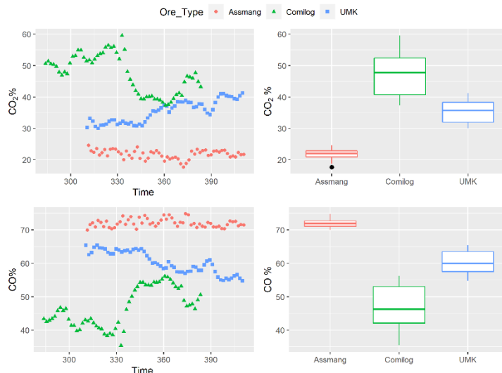
Figure 5: Off-gas composition for time region 300 - 400 minutes (left) and the corresponding average values (right) for Comilog, UMK and Nchwanning (Assmang) pilot experiments
