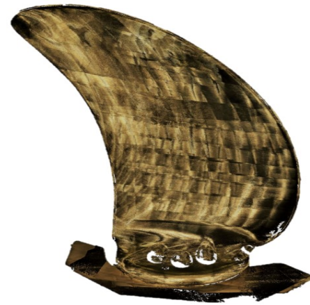
(b) The resulting point cloud after inspection of the propeller blade surface.
