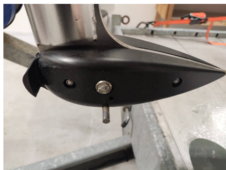
(b) Side view of the strut extremity, where the hydrofoil was connected.
